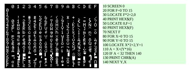
Figure 4.1 – Complete ASCII table from Gradiente Expert MSX 1.
