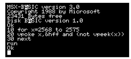
Figure 3.1. Inverting the colors of the character "A".
